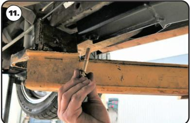
**11.** Install a 3/8" flat washer on a 3/8"-16 x 2 1/2" hex bolt. Insert the bolt/washer in the inner hole of the subframe connector. This hole goes through the tube of the subframe connector and lines up with the u-nut that is in the OEM frame rail. Thread the bolt into the u-nut. Leave the hardware loose until later.
