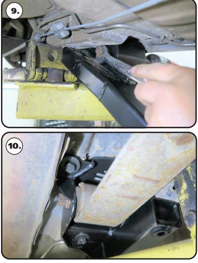
**9.** Attach the rear of the subframe connector to the front of the leaf spring. Install the leaf spring bolt from the inside of the car with the nut to the outside. The leaf spring bolt will need to be tightened before the subframe connector is installed.
