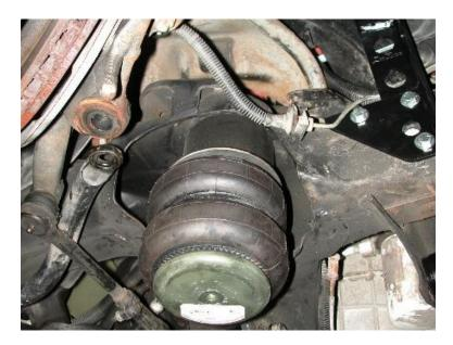
**Note:** If using a stock style sway bar, the end link spacer may need to be shortened 1.5" to attain proper clearance between the sway bar and the outer tie rod.
