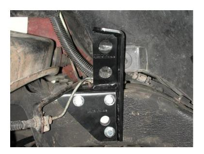
1. The shock bracket must be mounted first. It bolts right behind the upper arm and locates off the large hole in the frame and in the bracket. The brake line bracket must be removed and then reinstalled over the top of the shock bracket. The shock bracket is secured with 1 ½" x 3/8" bolts with Nylok nuts and flat washers.
