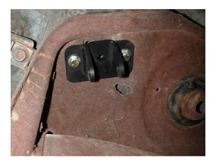
5. Fasten the new upper shock bracket into the factory shock location using the 5/16" x 1" bolts, flat washers and Nylok nuts supplied.
