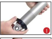
First using the supplied lower adjuster nut(90002222) thread the nut onto the shock from the bottom side as seen in figure 1
