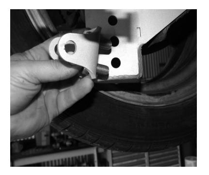
8. Install the Lower Bolt on Shock Bracket in the top 2 holes using (2)  $\frac{1}{2}$ " x 1  $\frac{1}{2}$ " Hex Bolts, and (2)  $\frac{1}{2}$ " Nylok Nuts.
