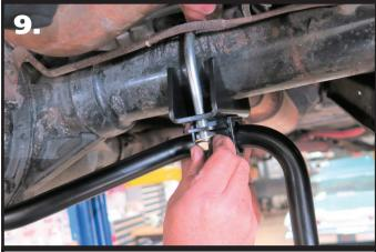
**9.** Hold the SwayBar in position on the car with the center bend toward the ground. Install a 7/16" Flat Washer & 7/16"-20 Nylok Nut on the threads of the u-bolts. Snug the hardware down and verify that it is centered and the axle mounts are level. Torque the u-bolt hardware.
