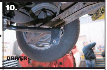
**10.** Thread (2) 3/8"-16 x 7/8" Socket Head Cap Screws into each of the Clamp-On Ends. Install a clamp-on end on each end of the bar. The End Link mounting hole should be mounted to the inside of the bar and pointing down. Start with the mount flush with the end of the bar.
