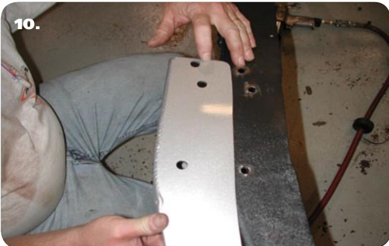
10. The original shock crossmember holes will line up with the holes in the "C" Notch. You can use these holes to double check your Notch placement.
