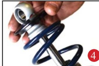
Slide the Derlin washer over the spring, Next slide the upper spring mount (90002222) over eyelet as seen in figure 4.
