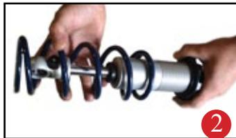
Next install delrin washers then coil spring over the top of the shock as seen in figure 2
