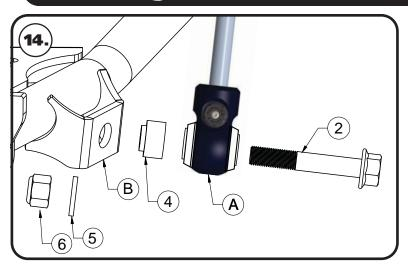
**14.** Attach the shock(A) to the lower control arm(B). Insert the 1/2"-20 x 3" flanged head bolt(2) through the bushing sleeve. Install the aluminum t-spacer(4) on the threads of the shock bolt with the SMALL OD toward the control arm. Insert the shock bolt/shock through the holes in the control arm shock mount. Install the flat washer(5) on the threads, followed by the 1/2"-20 nylok nut(6). Torque the nut to 75 ftlbs.
