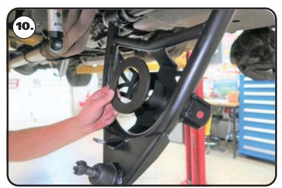
**10.** Use the guide on **Page 3** to determine what shims, if any, to use to achieve the desired ride height. Place the shims over the center ring. They will sit flat against the floor of the control arm.
