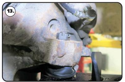
**13.** Slide the ball joint pin into the spindle and install the castle nut. Torque the ball joint nut and install cotter pin.
