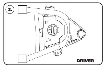
**2.** The control arms are marked "D" for Driver and "P" for Passenger. The ball joint pin points up and the sway bar mount is on the front side of the arm. **Image 2** shows a top view of the driver side control arm.
