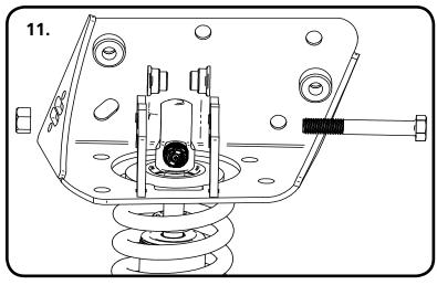
**11.** Install a spacer on each side of the upper Shockwave/Coilover. Slide the assembly into the upper mount from the bottom side. If your shock has an adjuster knob position it to the wheel side of the mount. Line up the hole in the spacers with the hole in the strap and insert 1/2" x 3 1/4" bolt and install 1/2" Nylok nut.
