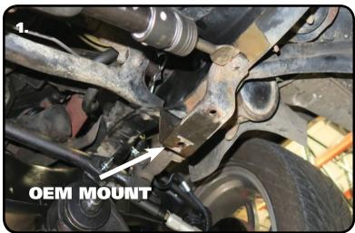
1. Some trucks are equipped with sway bar. If your truck has one, the OEM mount will need to be removed to install the StreetGrip Sway Bar. This is done by removing the rivets. The rivets can be removed by chiseling the heads off and driving them out or by drilling the rivets out. The new Frame Mount bolts directly in place of the old mount. If your truck doesn't have a sway bar, the mounting holes will still be in the frame.
