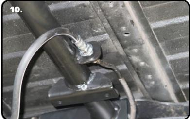
**10.** Attach the rubber brake line to the Upper Cross Member using the OEM clip. You may have to tweak the steel brake line to reposition it to thread into the rubber brake line. Thread the steel brake line into the rubber brake line and tighten.
