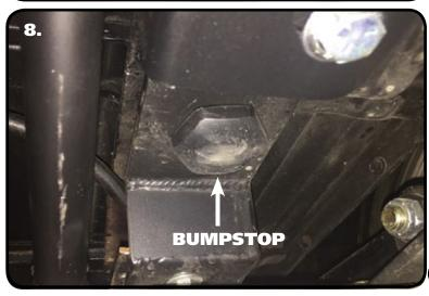
**8.** Install the bumpstops into the "C" Notches using a 3/8" nut and flat washer. Tighten the hardware enough to hold the bumpstop in place.
