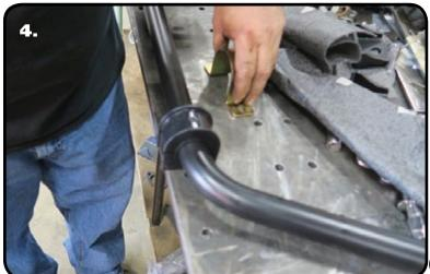
**4.** Open up the Poly SwayBar Bushings and install them over the Delrin Sleeves.
