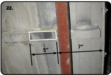
**22.** To allow clearance for the C-Notch, a section of the bed floor brace that is above the axle must be removed. This section is approximately 5" wide and about 7" from the fender well.
