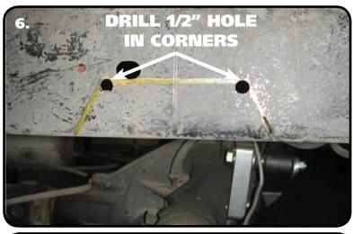
**6.** Use the supplied Template to mark the cut lines on the frame, then drill out the two corners with a ½" drill bit. This will give the cut a round edge and eliminate the possibility for stress fractures. Then cut the notch with a saw-z-all, cutoff wheel or plasma cutter. Grind all edges smooth.
