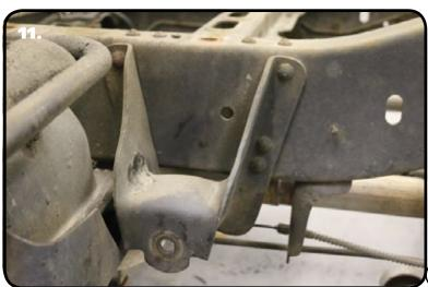
11. The OEM front leaf spring mounts will need to be removed from the frame rail. This can be done by either drilling the rivets out or removing the rivet heads and driving them out. We remove the rivet heads by cutting a " + " in the head with a die grinder then we cut the head off with a hammer and chisel or with an air chisel. Once the head is removed, the rivet can be driven out with a hammer and punch. After removing the frame mounts, drill the rivet holes with a 7/16" drill bit.
