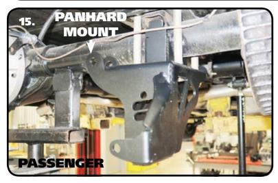
**15.** Repeat the above step on the Passenger Lower Mount. Torque the hardware to 60 ftlbs in a crisscross fashion.
