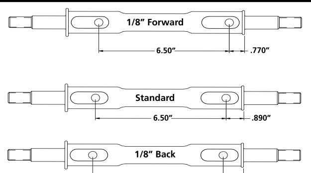
These StrongArms come equipped with a changeable caster slug setup. This allows you to add or remove caster from the front suspension, if desired. The caster slugs that come supplied in the kit are setup to provide approximately 5 degrees of caster. The caster slugs allow you to add or remove caster without having to use a stack of shims. If more or less caster is desired, optional slugs can be purchased from Ridetech or your Ridetech dealer.
