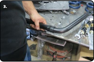
**3.** The Delrin Liner is split on one side to ease installation. We found it easier to install by opening up the Liner enough to slide it onto the end of the SwayBar, then sliding it into position. It will open up and slide over the curves in the Bar. Install a Liner on each side of the SwayBar in the approximate location they will need to be when installing the SwayBar on the Truck.
