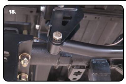
**18.** Install the Panhard bar into the frame bracket. The Panhard Bar is a bent bar, it is bent to clear the center section of the rear differential. The bar needs to be mounted with the BEND to the REAR, this will help it clear the differential cover. The Panhard bar is attached using (1) 5/8" x 3" bolt, (1) 5/8" Nylok Jam Nut & (2) 5/8" Flat Washers. Tighten the hardware enough to eliminate any gaps.
