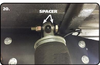
**20.** Insert a Spacer into each side of the upper Shockwave/CoilOver bearing. Slide the assembly into the upper shock mount. If your shock has an adjuster knob, position it so that the knob points toward the outside of the truck. Line up the hole in the spacers with the hole in the upper shock mount and insert 1/2" x 2 1/2" bolt and 1/2" Nylok nut with a 1/2" SAE Flat Washer on each side of the mount.
