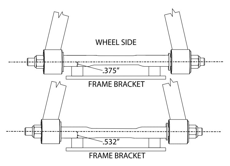
The cross shaft that is used in the upper control arms is offset. The offset combined with the caster slug option allows you to achieve the alignment setting you desire with minimal shims. To change the direction the Icon faces simply spin the cross shaft in the control arm.
