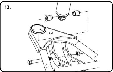
**12.** Install a spacer on each side of the lower Shockwave/Coilover. Slide the shock with the spacers installed into the lower control arm. Raise the arm up to line up the holes in the bushing with the 1/2" hole in the control arm straps and hold it in place while you install the 1/2" x 3 1/4" bolt and 1/2" Nylok nut. Tighten the upper and lower shock bolts to 75 fltbs.
