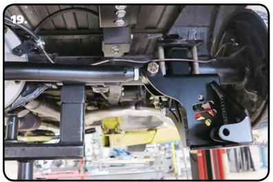
**19.** Install the other end of the Panhard bar into the mount on the Passenger Lower Axle Mount. The Panhard bar is attached using (1) 5/8" x 3" bolt, (1) 5/8" Nylok Jam Nut & (2) 5/8" Flat Washers. Tighten the hardware enough to eliminate any gaps.
