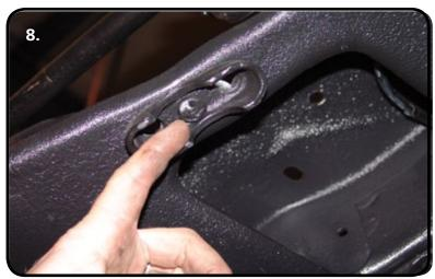
**8.** The lower control arm is installed using the factory U-bolts and nuts. The lower control arm is located by a pin that is in the center of the front u bolt cradle. This pin will go into the hole in the control arm shaft to help locate the control arm.
