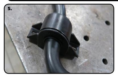
**5.** Install Bushing Straps Over the Poly Sway-Bar Bushings.
