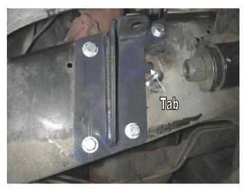
1. Place the new upper shock mount against the frame, the tab in the front of the bracket will slide into the factory shock stud hole. Position the bracket so that the bottom of the bracket is parallel to the bottom of the frame. Using the bracket as a template, mark an drill four 3/8" holes in the frame rail. Secure the bracket to the frame using four 3/8" x 1 ½" bolts, Nylok nuts and flat washers.
