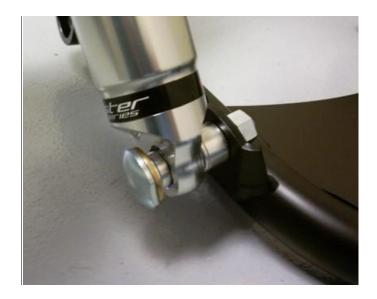
3. Attach the shock to the lower control arm using the cantilever pin supplied. See diagram on following page.
