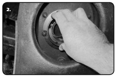
2. The Upper Coil Spring Seat is notched for a Rivet in the OEM Seat. The Notch MUST be lined up with the Rivet when installing the CoilSpring/Seat Combo.
