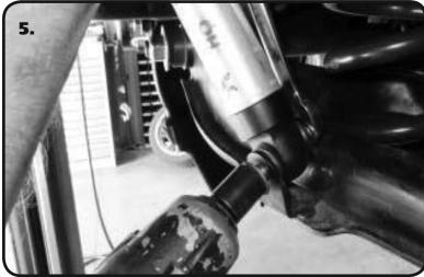
**5.** Jack the control arm up to seat the Coil-Spring and attached the bottom of the shock.
