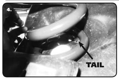
**4.** Insert the CoilSpring/Seat combo into the OEM coilspring pocket aligning the Rivet in the notch of the Upper Seat. Twist the spring on the Upper Seat to get the bottom of the CoilSpring lined up with the receiver in the control arm. The end of the CoilSpring needs to be nested into the receiver area of the Control Arm.
