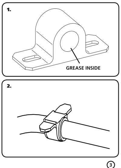
**1.** Apply Lithium grease to the inside of the sway bar bushings using the tube of grease supplied in the kit.
