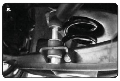
9. SWAYBAR CONTROL ARM **8.** Install a 3/8" Flat Washer on (2) 3/8"-16 x 1 1/4" Hex Bolts and insert them into the holes. Install a 3/8" Flat Washer and 3/8"-16 Nylok Nut on each Bolt. Repeat on the other side and tighten hardware.
