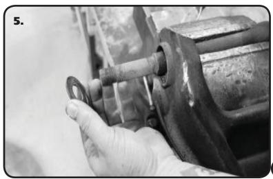
5. UPPER CONTROL ARM: The Upper Control arm has an inner washer on the cross shaft that needs to be removed before installing the Delrin Bushings.
