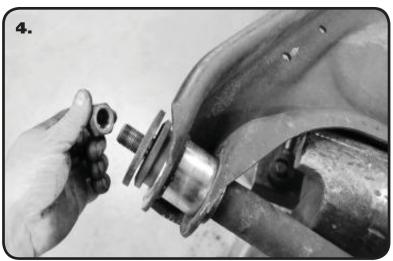
**4.** Insert the cross shaft into the control arm by sliding it through the Outer Shells installed in the arms. Push the Inner Sleeve into the Delrin Bushing. Push the Delrin Bushing/Inner Sleeve assembly into the Outer Shells. They will go in partially. Install the OEM washer and nut on each end of the cross shaft. Tighten the Hardware on each end until the Delrin Bushings are bottomed out against the lip of the Outer Shell installed in the control arm.
