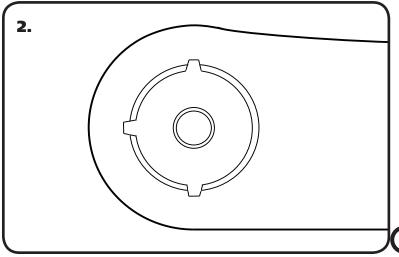
2. The OEM bushings in the Lower Control arm are staked outward. These Staked areas will need to be knocked inward to be able to remove the bushings. This can be done with a hammer and chisel. Knock the areas in far enough that the will clear the inside diameter of the bushing hole.
