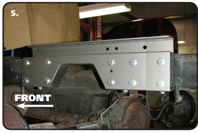
**5.** Slip the C-Notch over the frame rail. Use the C-Notch as a template to drill the (10) holes in the side and (3) in the bottom. Use a 1/2" drill bit to drill the holes. Install a 1/2" Flat Washer on each of (10) 1/2"-13 x 1 1/2" Bolts. Insert a bolt/washer in each hole. Install a 1/2" Flat Washer and 1/2"-13 Nylok Nut on the threads of each bolt/washer and tighten. Torque the hardware to 75 ftlbs.
