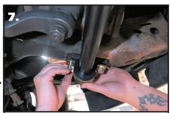
**7.** Slide the SwayBar into position on the truck with the SwayBar arms above the tie rods. Install a Lock Washer & Flat Washer on the each M10 Hex Bolts. A 30mm goes in the front, with a 40mm going in the rear. Do **NOT** complete tighten the hardware at this time.
