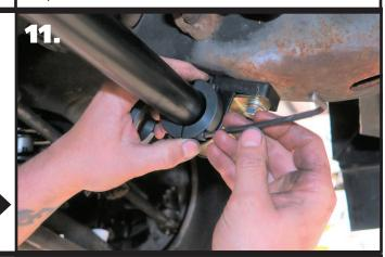
**11.** Center the swaybar and torque the strap hardware. Install the stop rings against the swaybar bushing. The stop rings will go against the inner side of the bushing. Take the stop rings apart and reassemble them against the bushing and tighten.
