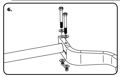
**6.** After the arms are installed, insert (2) 5/16" x 2 3/4" bolts with a 5/16" washer on each, through the Clamping Holes in the Arms. Install a 5/16" Flatwasher and 3/8" Nylok on the Bolt and Torque to 25 ftlbs. It will be necessary to torque each bolt multiple times.
