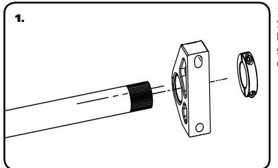
**1.** Install both Bushing Mounts onto the Splined Bar with the Flange side of the Inner Bushing facing out. With the Bushing Mount slid onto the bar, install the Locking Ring, but do not tighten.
