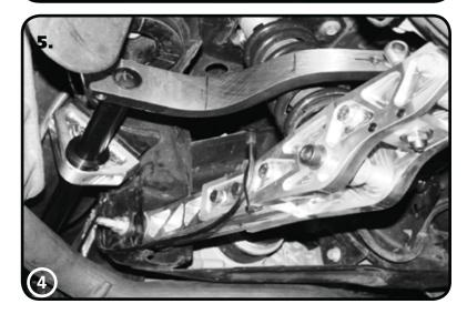
**5.** The PosiLink can be used to get the arms clocked the same. Install one Arm on the Drivers Side and rotate it up and down until you can insert the PosiLink in the center hole. On the Passenger Side, install the arm on the Sway Bar. Try to insert the PosiLink in the center hole. Remove the Arm from the Splines and move it one Tooth at a time, reinstalling the arm until the PosiLink will go in the center hole easily.
