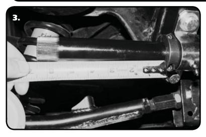
**3.** Center the Splined Bar by measuring each side and sliding it in the mounts until both sides measure the same. Once the Splined Bar is centered, tighten the Mounting Blocks. Next, slide the Locking Ring up against the Bushing and tighten the Locking Ring.
