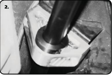
**2.** Bolt the assembly into the OEM Swaybar location, with the LONG SIDE UP, using (4) 5/16" SAE Flatwashers, (4) 8M Lockwashers and (4) 8M-1.25 x 50mm Hex Bolts. The mounts are bolted with the long side on the top. Run the bolts down until they touch, but DO NOT TIGHTEN.
