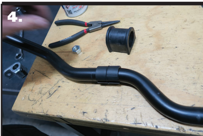
4. Install the Delrin Liner by sliding it over the end of the bar into position. Position it in the area that the bushing will ride based on the location of the stock swaybar. Do this on both ends of the swaybar.
