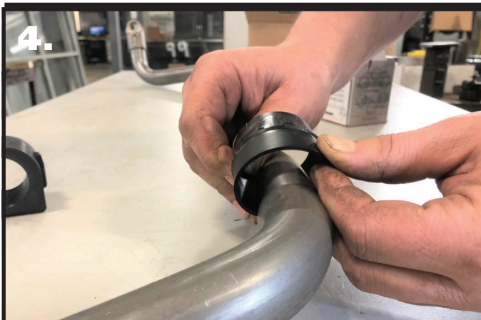
4. Open the Delrin Liner at the split and slip it over the SwayBar. Position it in the area that the bushing will ride based on the location of the stock swaybar. Do this on both ends of the swaybar.
