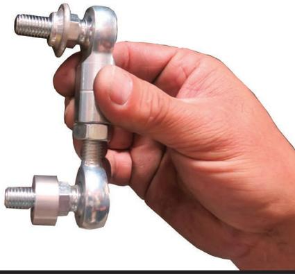
**17.** Install a T-bushing on one end of the linkage (small diameter out), with a .300" thick spacer on the other end. The end with the T-bushing will be the TOP end of the linkage that will be installed in the swaybar end.
