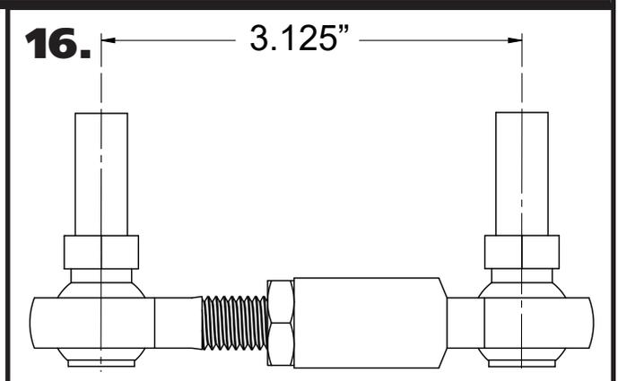
**15.** Assemble the end links. First, thread a M10-1.5 Jam Nut onto the threads of the male endlink body. Next, thread the male endlink body into the female endlink body. Set them to 3 1/8" center to center of the endlinks. Keep the end links parallel with each other and tighten the jam nut against the female endlink.
