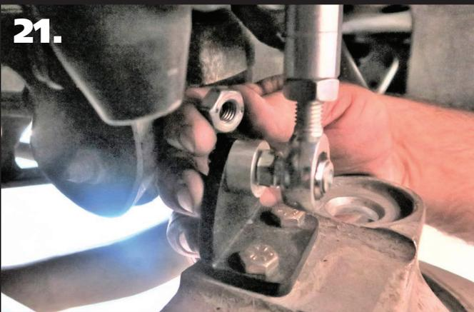
**21.** Install a M10 flat washer and M10-1.5 serrated lock nut on the threads of the lower stud of the linkage. Repeat Steps 15-20 on the other side. Torque the hardware to 37 ftlbs.
