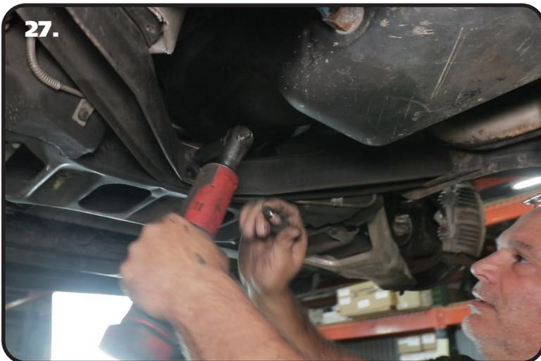
27. Reinstall the crossmember brace if working on a later model Corvette.
