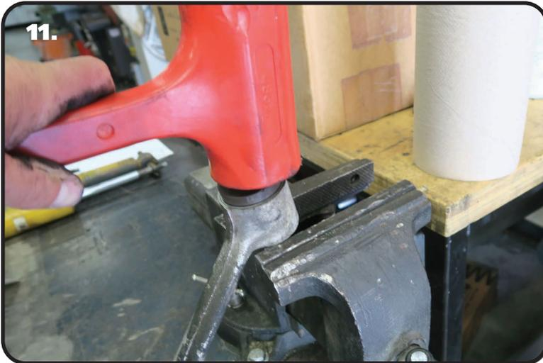
**11.** Tap the bushing/sleeve into the control arm. Support the inside of the control arm, but make sure the opening is large enough for the control arm bushings to pass through.
