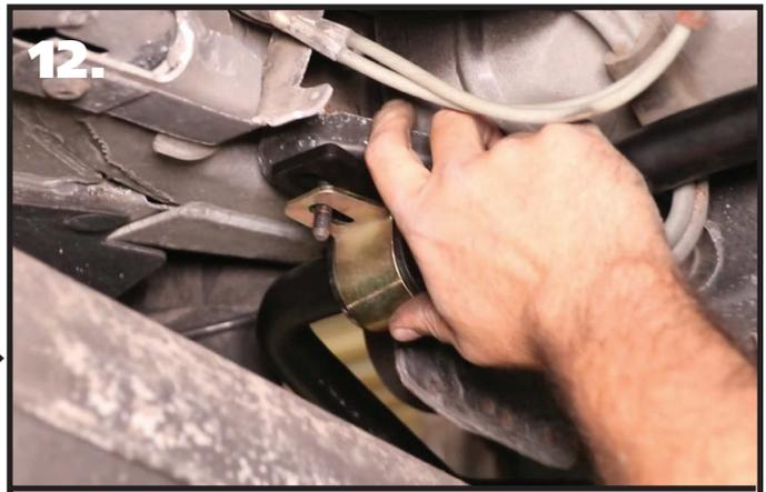
**12.** Install the bushing spacers under the swaybar bushings. They need to be installed with the bolt holes offset towards the wheel. The spacers will slide over the OEM mounting studs.
