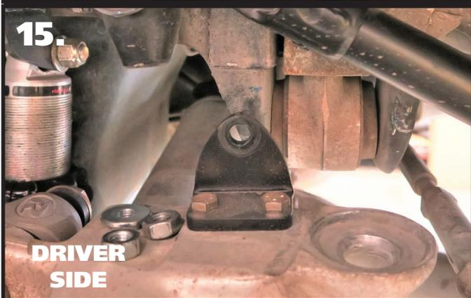
**15.** Install the new linkage mounts in place of the OEM mounts. They are installed with the mounting holes to the wheel. Line up the mounting holes with the OEM holes. Install a 5/16"-18 x 1 1/4" bolt, flat washer, and 5/16"-18 nylok nut. Torque hardware to 25 ftlbs.
