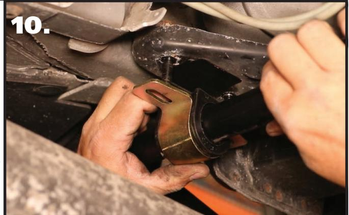
**10.** Install the Bushing Straps on the swaybar bushings. They need to be installed with the bolt holes offset towards the wheel.
