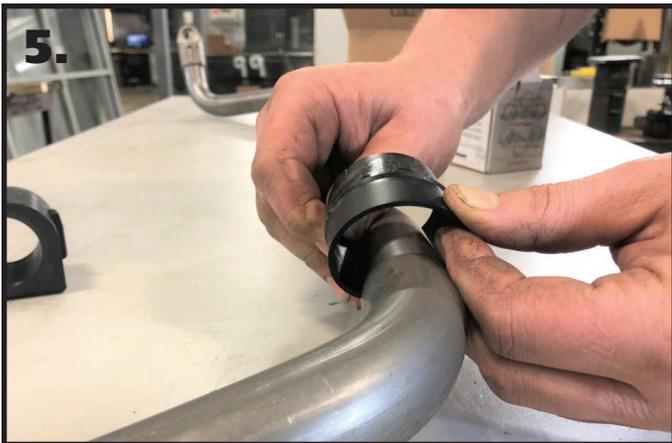
**5.** Open the Delrin Liner at the split and slip it over the SwayBar. Position it in the area that the bushing will ride based on the location of the stock swaybar. Do this on both ends of the swaybar.
