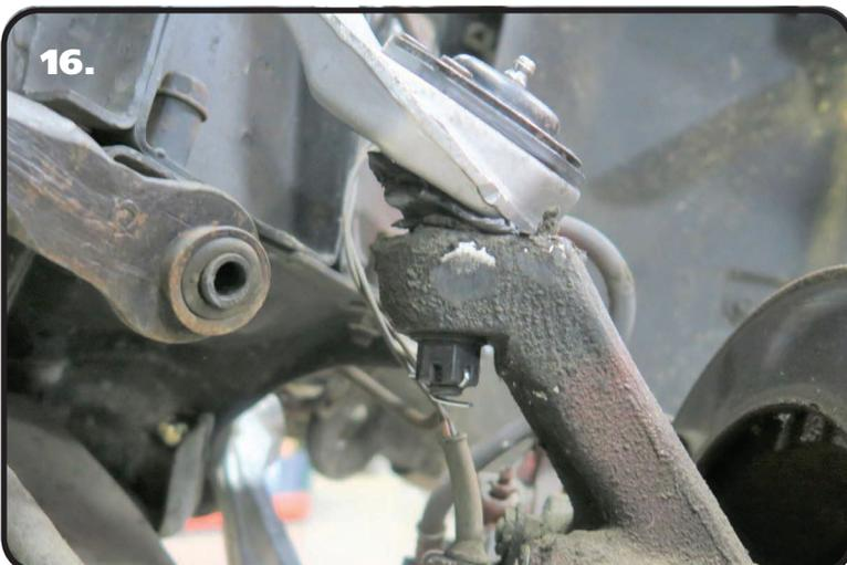
**16.** Insert the upper ball joint into the spindle. Reinstall the castle nut and torque to 33 ftlbs. Check alignment of the cotter pin hole. If it does not line up with an opening in the castle nut, tighten the nut until it does line up. Reinstall the cotter pin and bend the ends to keep it in place.
