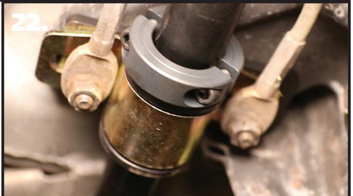
**22.** Disassemble the Locking Rings provided in the kit. The locking rings will need to be installed against the inside edge of the swaybar bushings. Assemble each locking ring against the swaybar bushing and tighten.
