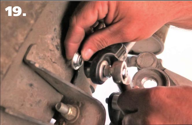
**19.** Install a 2nd T-bushing on the threads of the upper stud with the small diameter sticking into the swaybar end.
