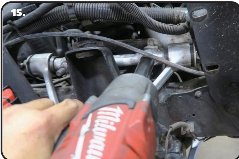
**15.** Reinstall the upper control arm. Make sure the upper mounting bolts are seated in the frame. Reinstall the shims stacks that came out of the car. Torque the nuts to 37 ftlbs.
