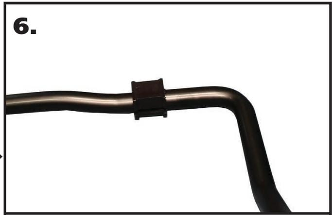
**6.** Open the SwayBar Bushing at the split and slide it **OVER** the Delrin Liner. Do this on both Delrin Liners.
