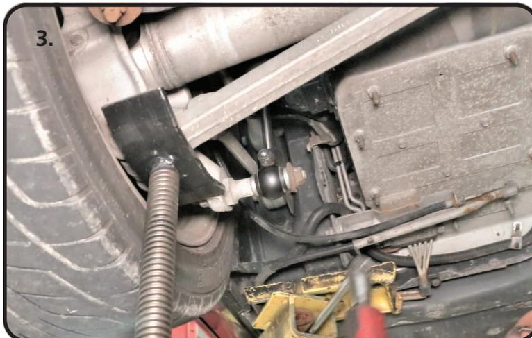
**3.** With the upper Shock installed, attach the lower eyelet of the shock to the OEM shock stud. Use the OEM hardware to attach the shock.
