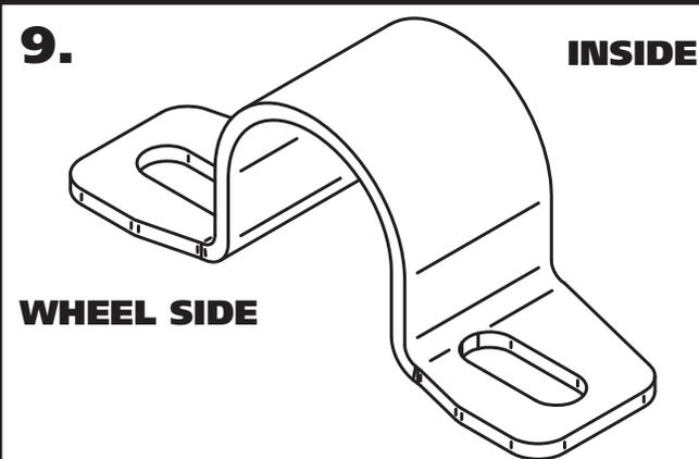
**9.** The bushing straps included in this kit are offset. The straps need to be installed on the car with the bolt holes offset to the wheel side of the bushing strap.
