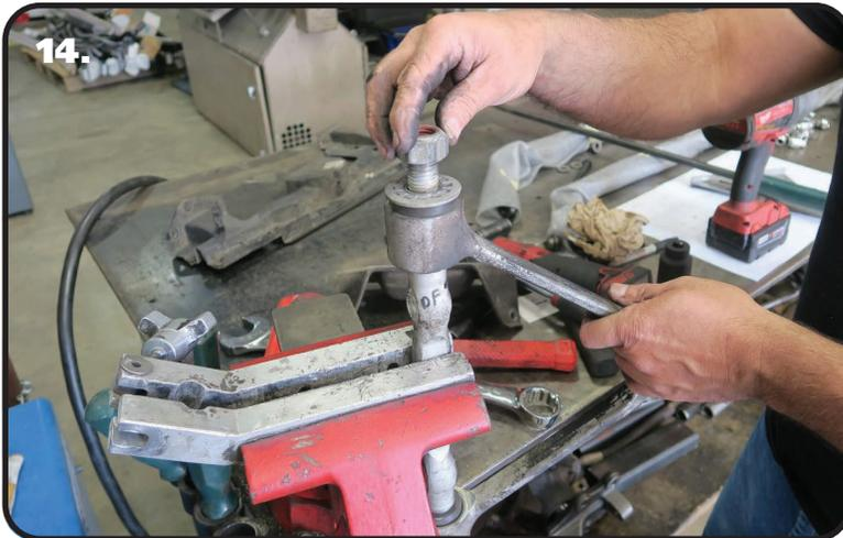
**14.** Reinstall the OEM outer washers and nuts. Torque the nuts 35-40 ftlbs.
