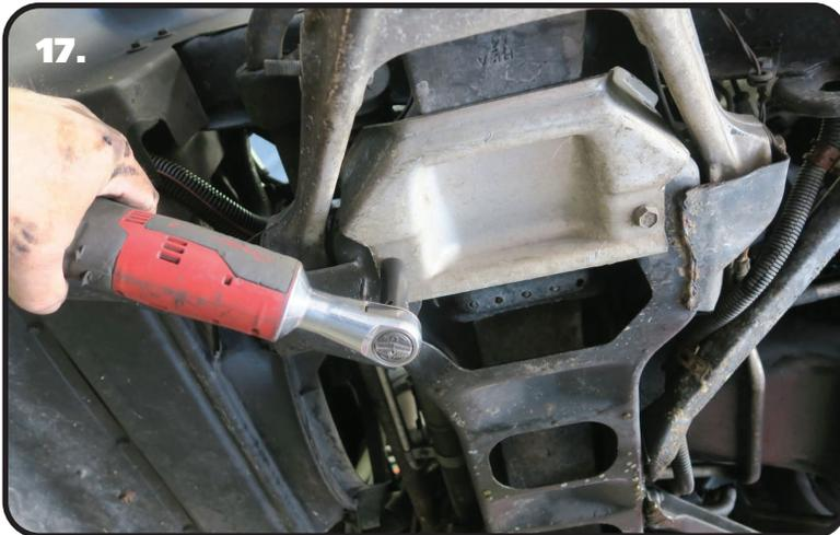
**17.** The spring travel limiter will need to be removed. There are 2 vertical bolts and 2 horizontal bolts.
