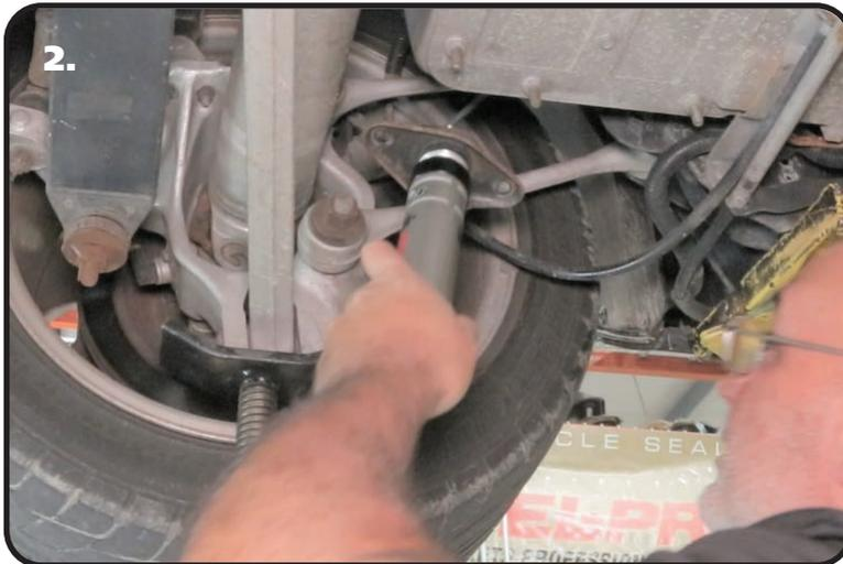
**2.** Install the shock/upper mount in the car. It will be reattached using the OEM hardware. Torque the hardware to 37 ftlbs.
