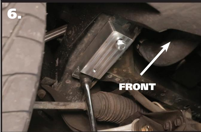
**6.** Bolt the Aluminum Spacer Block to the frame. The spacer bolt is attached to the frame using a M10-1.5 x 40 bolt and M10 flat washer in the rear hole. A M10-1.5 x 60mm bolt will be used in the front hole for alignment purposes. Torque the rear bolt. Remove the front bolt, it will get reinstalled later.
