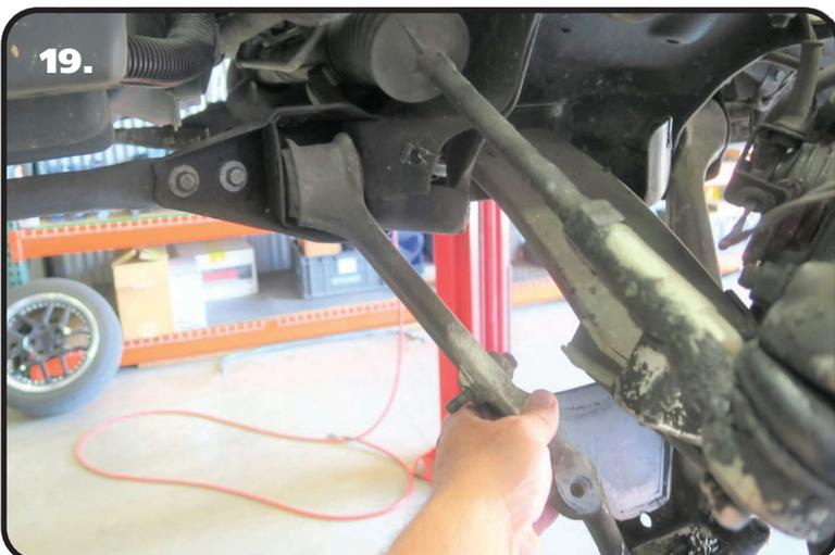
**19.** Support the hub/spindle and separate the ball joint from the spindle. With the ball joint separated, remove the control arm bolts and the control arm.
