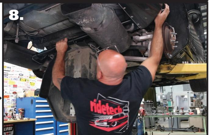
**8.** Slide the swaybar in place. The rest of the exhaust may need to be pulled down to get the swaybar installed.
