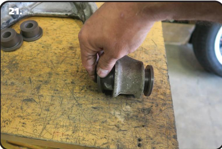
21. Insert a bushing half in each opening of the control arm. The front and rear bushings are the same size.
