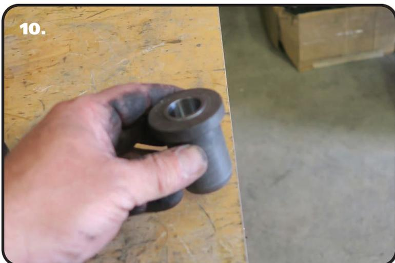
10. Install the Inner Sleeve in the upper control arm bushings. You can tap it in with a hammer or use an arbor press. The front upper bushings are 2 different sizes with the front bushing being the larger of the 2. Make sure you have the correct bushings for the location.
