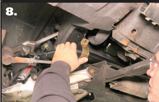
**8.** Install the Bushing Straps on the swaybar bushings.
