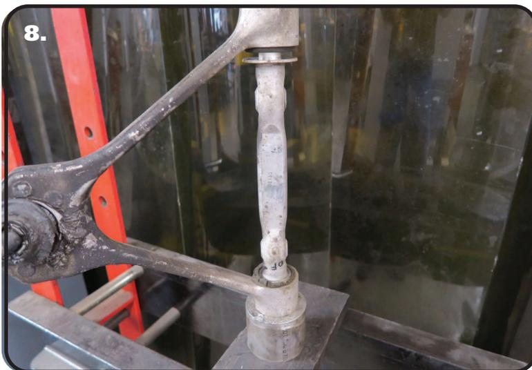
8. Remove the outer nuts and washers and retain them. Press the bushings out of the control arm. We used a "H" press to remove ours. Use the cross shaft to push the bushings out. Push out the bushing with the small inner washer first. After pushing it out, the large inner washer can be removed from the cross shaft to be able to push the remaining bushing out.
