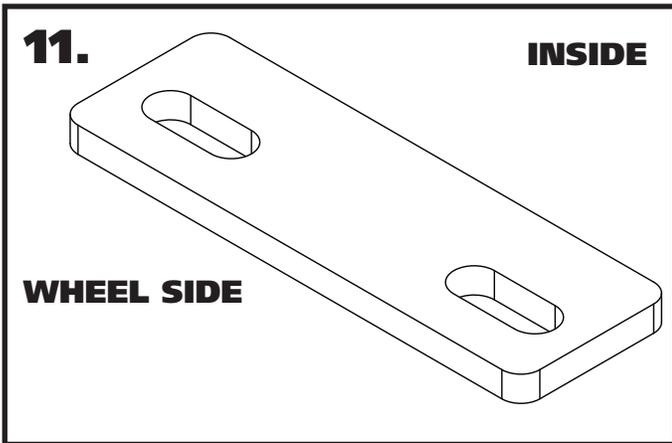
**11.** Just like the bushing straps, the bushing spacers included in this kit are offset. The bushing spacers need to be installed on the car with the bolt holes offset to the wheel side of the bushing strap.
