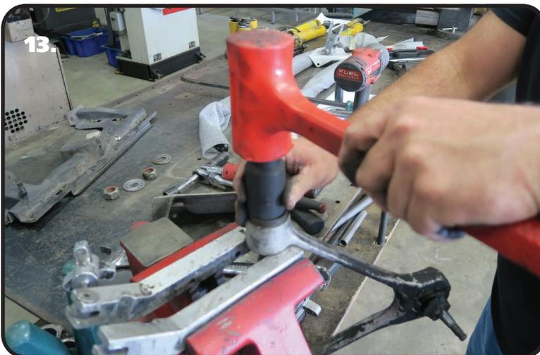
**13.** Tap the remaining bushing into the control. To do this, support the inside of the control arm. Again, make sure the opening is wide enough for the bushing to pass into it. We used a large deep well socket to tap the bushing in.
