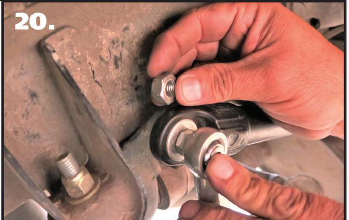
**20.** Install a M10-1.5 serrated lock nut on the threads of the upper stud of the linkage.
