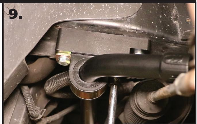
**9.** Bolt the bushing straps in place using (1) M10-1.5 x 60mm hex bolt and M10 flat washer in the front hole. The rear holes uses (1) 3/8"-16 x 1" bolt and M10 flat washer. Insert the hardware through the bushing strap bolting the strap in place. **DO NOT TIGHTEN THE HARDWARE** at this time.
