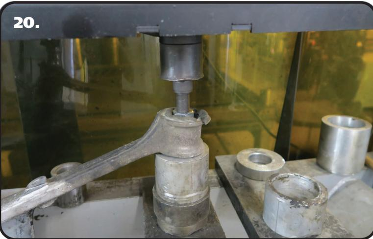
20. Press the bushings out of the control arm. We used a "H" press to remove ours. Once the Bushing Assembly is removed from the arm, prep the bushing opening by cleaning it to remove any debris that may be left in the opening.
