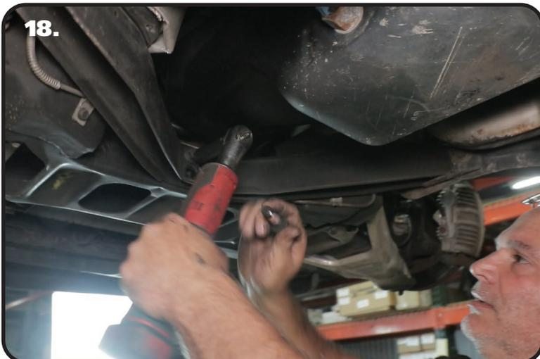
**18.** Later cars have a brace on the back side of the crossmember that will need to be removed to allow for removal of the rear control arm bolt. Remove the nuts from the lower control arm bolts to prepare for control arm removal.
