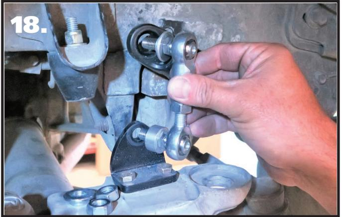
**18.** Install the Linkage with the Studs pointing to the center of the car. The linkage will be installed with the previously installed t-bushing in the swaybar end.
