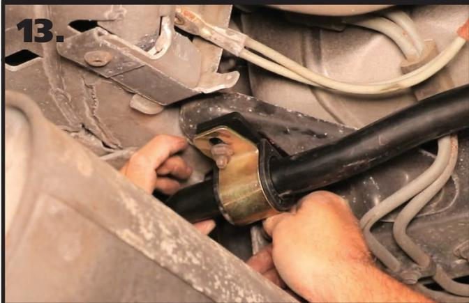
**13.** The swaybar bushings/straps will slip in place on the OEM studs. Push the swaybar up in place. Reuse the OEM hardware to attach the swaybar bushings/swaybar to the car. Torque nuts to 18 ftlbs.
