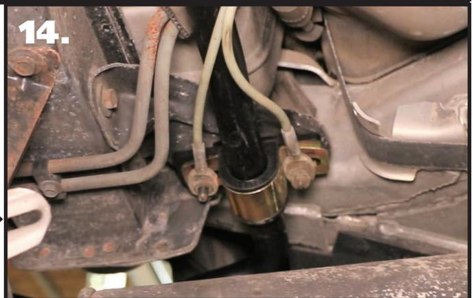
**14.** Use the OEM hardware to reattach the gas tank safety cables to the swaybar mounting studs.
