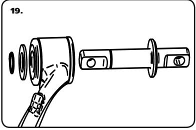
**19.** Install a Trunnion into each set of Bushings installed in the Control Arm. The Trunnions are inserted with the Shoulder to the outside of the Control Arm. Install a 3/4" Washer followed by a Snap Ring on each Trunnion.
