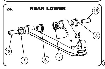
**24. Rear Lower -** Using the Diagrams on Page 2 & 3, Insert the correct Bushings in the correct locations using a Bench Vise to push them in. Push the Bushings in followed by the correct Inner Sleeve. The Front Lower uses Bushing[5,6,7,8], and Inner Sleeve[18].
