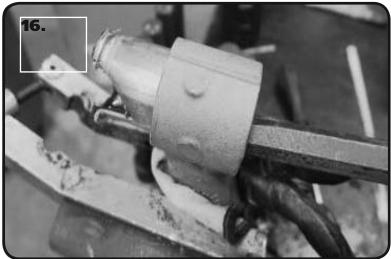
**16.** Once the bushing starts moving, knock it the rest of the way out. This will leave you with a clean inside bore that is ready for a Delrin Bushing to be installed.
