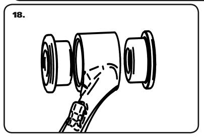
**18.** Press a set of bushings into each opening of the upper control arm. A bench vise can be used to do this.
