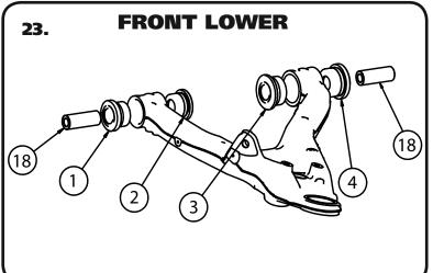
**23. Front Lower -** Using the Diagrams on Page 2 & 3, Insert the correct Bushings in the correct locations using a Bench Vise to push them in. Push the Bushings in followed by the correct Inner Sleeve. The Front Lower uses Bushing[1, 2, 3, 4], and Inner Sleeve[18].
