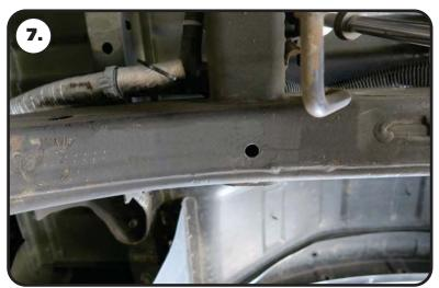
**7. Image 7** shows the drilled hole to help give you an idea of the position. Hold the bracket on the bottom of the frame rail and mark the hole to be drilled. Again, the bracket needs to be centered below the crossmember with the locating tab against the outside of the frame rail.
