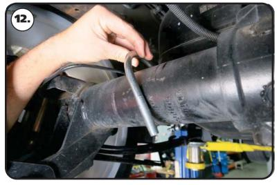
12. Install a 7/16" u-bolt on each axle tube
