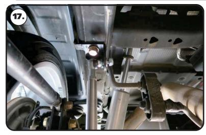
**17.** Install a M10 flat washer & M10-1.5 nylok nut on the threads of the PosiLink Torque the nut to 37 ft-lbs. Repeat on the other side.
