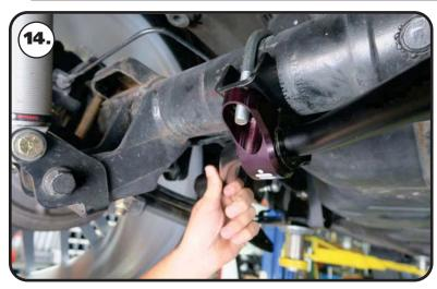
**14.** Hold the sway bar in position on the truck with the center bend toward the ground. Slide the sway bar bushing strap onto the u-bolt.
