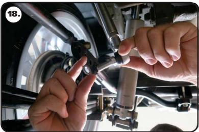
**18.** Install a M10 flat washer on the threads of the PosiLink. Insert the PosiLink in the **MIDDLE** mounting hole of the sway bar arm. The threads of the PosiLink should be pointing to the outside of the truck.
