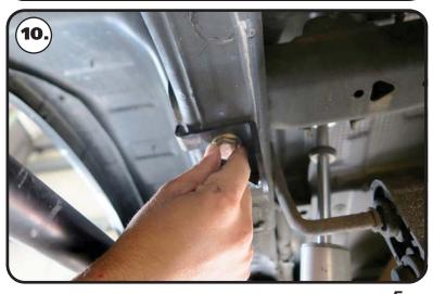
**10.** Install a 1/2" flat washer on a 1/2" - 13 x 2 3/4" bolt. Hold the frame bracket in place with the tab on the outside of the frame. Insert the bolt/washer in the aligned holes.
