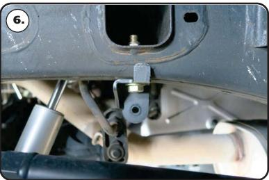
**6. Image 6** shows the passenger side frame bracket installed. The frame/crossmember will need to be drilled with a 1/2" drill bit. The frame bracket is centered below the crossmember with the locating tab against the outside of the frame rail.
