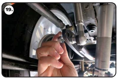
**19.** Install a M10 flat washer & M10-1.5 nylok nut on the threads of the PosiLink Torque the nut to 37 ft-lbs. Repeat on the other side.
