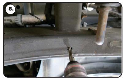
**8.** Drill the bottom of the frame with a 1/2" drill bit.
