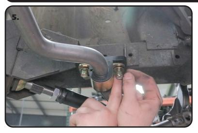
**5.** Slide the sway bar into position on the car. The sway bar arms will be bending upward with the center dropping toward the ground. Install a 3/8" flat washer on (4) 3/8"-16 x 1 1/4" hex bolts. A bolt/washer will go in each of the 4 mounting holes. With the bolt/ washers installed, install a 3/8" flat washer on the threads followed by a 3/8"-16 nylok nut. Do **NOT** completely tighten the hardware. It will be left partially loose until the end links are installed.
