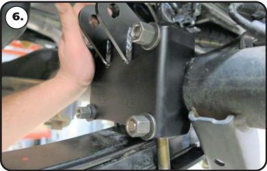
**6.** Install a 1/2" flat washer & 1/2"-13 nylok nut on the threads of the u-bolts. Snug the hardware down to eliminate and play in the hardware, but leave loose enough to rotate the mount on the axle tube. Rotate the mount upward until it stops against the leaf spring pad. Torque the nuts to 55 ft-lbs in a criss-cross fashion. Repeat on the other side.
