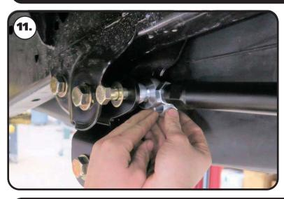
**11.** The front heim requires a .825" spacer on each side of the heim to position it in the front bracket. Install a 5/8" flat washer on a 5/8"-18 x 4" bolt. Start the bolt/washer in the outer tab of the front mount. Install a spacer on the bolt sticking through the outer tab. Slip the bolt into the heim and inert the 2nd spacer on the other side of the heim. Push the bolt all the way in and install a 5/8" flat washer and 5/8"-18 nylok nut. Torque to 115 ft-lbs.
