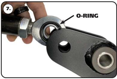
**7.** Install a supplied o-ring on each side of the rod end that will slip into the rear pivot. Hold the o-rings in place as you insert the rod end into the pivot.
