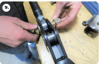
**9.** Install a 5/8" flat washer and 5/8"-18 nylok nut on the threads of the bolt. Torque to 115 ft-lbs. Repeat for the other side.
