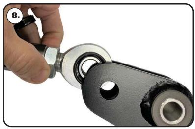
**8.** Align the mounting holes with the through hole of the rod end. Install a 5/8" flat washer on a 5/8"-18 x 2 1/2" bolt. Insert the bolt/ washer though the aligned holes. Assemble both bars & pivots.
