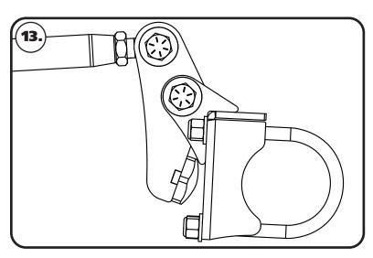
**13.** WITH THE TRUCK ON THE GROUND, THE SET LENGTH OF THE BARS NEED TO BE CHECKED. The bars need to be set so there is approximately 1/8" gap between the bumpstop and axle mount. Adjust the traction bar to get this gap set. After you check the gap, tighten the jam nuts on the traction bar.
