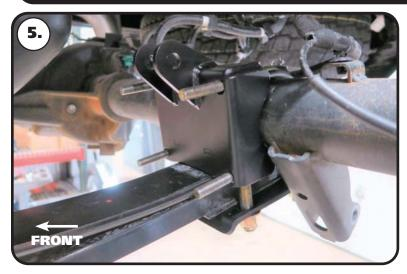
**5.** Slip the u-bolts over the axle with the threads pointed forward. They will locate on the outsides of the leaf spring u-bolts. Next, slip a traction bar mount over the u-bolts with the pivot mount at the top.
