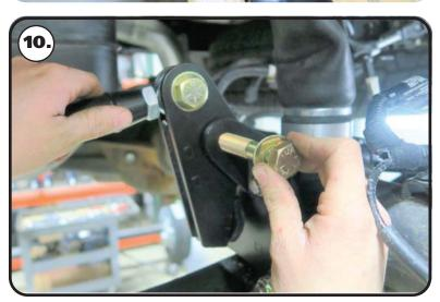
**10.** Insert the pivot/bar into the axle mount. The pivot needs to be installed with the bar at the top and the bumpstop to the axle mount. Install a 5/8" flat washer on a 5/8"-18 x 3 3/4" bolt. With the mounting holes aligned with the pivot inner sleeve, insert the bolt/washer. Install a 5/8" flat washer & 5/8"-18 nylok nut on the bolt. Torque to 115 ft-lbs.
