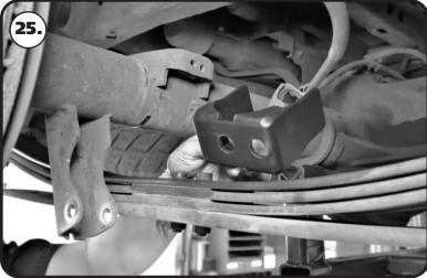
**25.** The flip bracket is positioned on the leaf spring locating pins. The locating pin holes will need to be positioned to the front of the truck.
