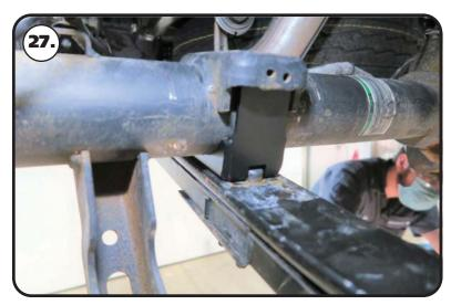
**27.** Slowly lower the axle into the flip bracket, making sure the tabs go up into the leaf spring saddle. THE FLIP BRACKET WILL POSITION THE PINION AT THE CORRECT ANGLE.
