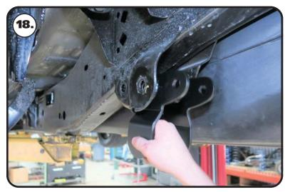
**18.** Insert the leaf spring hanger bracket into the OEM leaf spring mount. The long tabs will point to the front of the truck and insert into the OEM mount. Position the bracket so that the tube lines up with the OEM leaf spring mounting hole.
