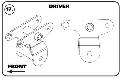
**17.** The kit includes brackets to relocate the front of the leaf spring. The brackets have a "D" or "P" stamped into the side of the bracket. The Driver side is shown in **Image 17**. The bracket is mounted in the truck with the cross tube to the top and the long tabs to the front of the truck.
