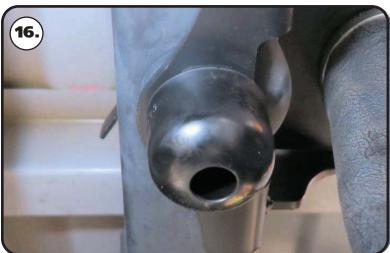
**16.** Install a M10 flat washer on a M10-1.5  $\times$  30 mm socket head cap screw. Insert the washer/bolt in the center hole of the bumpstop. Use a hex key (allen) wrench to attach the bumpstop in the OEM location. Repeat on the other side and torque to 28 ftlbs.
