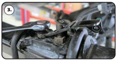
**3. 2021-2022 ONLY!** Disconnect the headlight sensor linkage from the Drivers side leaf spring mount. Remove the linkage bracket from the axle. There isn't a sensor on the Passenger side of the truck.
