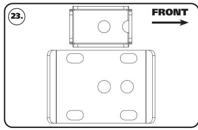
**23.** The flip kit has the locating holes offset to center the wheel in the wheel opening. **Image 23** illustrates a top view of the flip bracket and the leaf spring plate. Notice the HOLES are offset to the FRONT of the truck.
