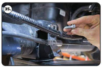
**35.** Remove the brake line bracket bolt from the rear of the drivers side leaf spring pad. Retain the hardware for assembly. If you are using the optional air springs, a longer bolt is supplied.
