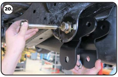
**20.** Make sure the holes in the front tab line up with the front hole of the OEM leaf spring mount. Install a 3/4" flat washer on a 3/4"-16 x 5" bolt. Insert the bolt/washer through the front hole of the leaf spring mount. Install a 3/4" flat washer & 3/4"-16 thin nylok nut on the threads of the bolt. Torque the hardware to 75 ftlbs.
