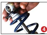
slide a Delrin washer over the eyelet. Next, slide the upper spring mount (803-00-199) over eyelet as seen in figure 4.
