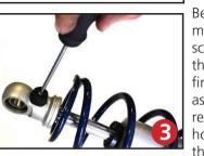
Before the upper spring mount can be installed screw the adjuster knob on the upper eye mount to the firmest setting (clockwise) as seen in figure 3. Then remove the Knob by holding it while removing the center screw.
