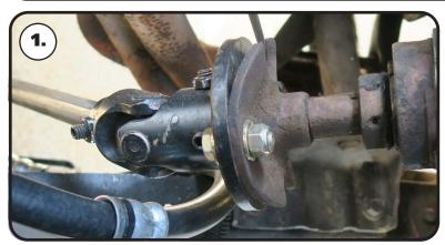
**1.** Align the (2) holes of the adapter with the (2) holes of the OEM column. Install a 5/16" flat washer on each of the (2) 5/16"-18 x 1" hex bolts. Insert the bolt/washers in the aligned holes. Install a 5/16" flat washer & 5/16"-18 nylok nut on each bolt. SNUG THE HARDWARE DOWN, BUT DO NOT TIGHTEN AT THIS TIME.
