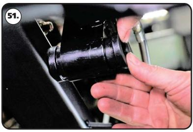
**51.** Insert the 2nd half of the rack bushings into the rack. Do this for each mount.
