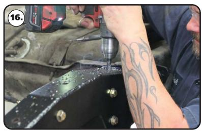
**16.** Use a 7/16" drill bit to drill the remaining holes in the top and bottom of the frame.
