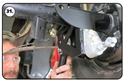
**31.** Insert (2) .625" ID x .740" long R-Joint spacers into the R-Joint of one end of each lower bar (23 1/8"). The small diameter of the spacer goes into the R-joint. Insert the rear lower bar R-Joint into the lower bar mount built into the axle mount.
