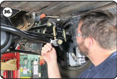
**36.** We used a die-grinder with a cutoff wheel to cut the brake line bracket off the axle tube. Be careful to not cut into the axle tube.
