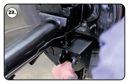
**23.** The kit includes a Driver and Passenger lower axle mount; the two are different. The Passenger mount has the panhard bar mount built into it. **Image 23** shows the Passenger mount. Hold the mount up in place against the bottom of the axle tube. The tabs will nest against the bottom of the leaf spring pad.
