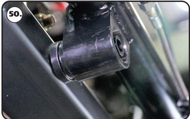
**50.** Install the rack on the bushing half. The steering shaft will be on the drivers side with the shaft pointing toward the cab.
