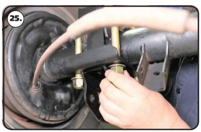
**25.** Hold the mount in place and install a 5/8" flat washer and 5/8"-18 nylok nut on the threads of the u-bolts sticking through the axle mount. Tighten the nuts evenly in a criss-cross fashion making sure the tabs of the axle mount are touching the leaf spring pad evenly. Torque the nuts in a criss-cross fashion to 75 ftlbs. Repeat on the other side.
