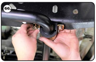
**66.** Install a 3/8" flat washer on each of (4) 3/8"-16 x 1 1/4" hex bolts. Hold the sway bar in place and insert a bolt in the mounting hole of the mounting strap. Install a 3/8" flat washer & 3/8"-16 nylok nut on the threads of the bolt. Repeat this on remaining mounting holes. Do NOT tighten the mounting bolts at this time. They need to left loose until the sway bar linkage has been attached to the lower control arm.
