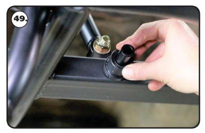
**49.** Install one half of a poly rack bushing on the rack mounting bung of the cradle. The bushing needs to be installed on the bung with the large diameter against the cradle. Install a bushing on each mounting bung.
