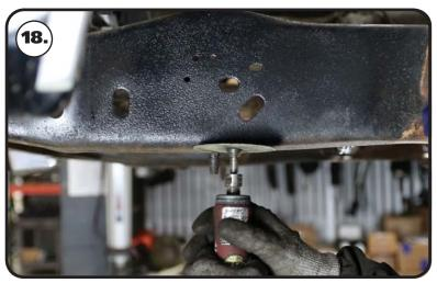
**18.** There is a pin that sticks down from the bottom of each frame rail that needs to be removed. These pins are in front of the OEM cross member. These need to be cut off even with the frame rail.
