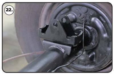
**22.** Sit the upper bar mount on the leaf spring pad of the axle. The locating pin needs to insert into the leaf spring locating hole of the leaf spring pad.
