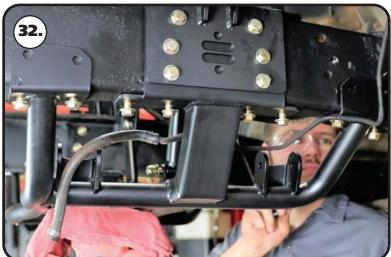
**32.** Install a 7/16" flat washer on each of (8) 7/16"-14 x 1 /4" hex bolts. Insert a bolt/washer in each bottom (8) holes. Install a 7/16" flat washer and 7/16"-14 nylok nut on the threads of the bolts. Again, snug the hardware down, but do not torque the hardware at this time. Do this for both sides.
