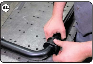
**63.** Open the sway bar bushing at the split and slip it onto the sway bar. Do this for both bushings.
