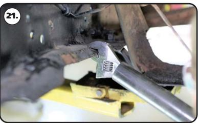
**21.** We used an adjustable wrench to bend the flange flat. Tighten the adjustable wrench tight to the rail and use the wrench to bend it upward. You will need to work up and down the frame rail bending it up to get the frame rail flat.
