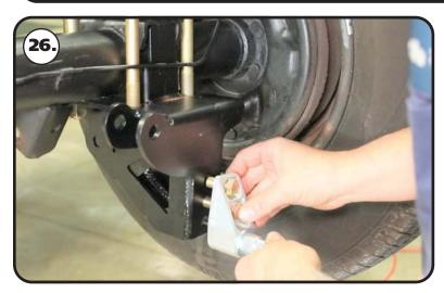
**26.** The lower shock mount attaches with (1) 1/2"-13 x 1 1/4" hex bolt, (1) 1/3"-13 x 1 3/4" hex bolt, & (2) 1/2" flat washer, & (2) 1/2"-13 nylok nuts. The lower mount gets attached to the 2nd and 3rd hole up from the bottom of the axle mount. When the shock mount is installed correctly, the bottom of the lower shock mount is 1/2" below the bottom of the axle mount. Insert the bolts through the aluminum shock mount with the 1 1/4" long bolt in the top hole, 1 3/4" in the bottom hole.
