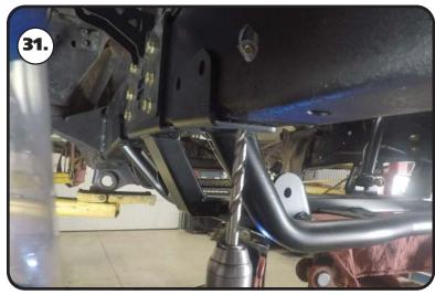
**31.** There are (8) mounting holes in the bottom mounts of each side of the cradle. All but (2) of these will need to be drilled with a 7/16" drill bit. (2) of the holes will align with factory holes.
