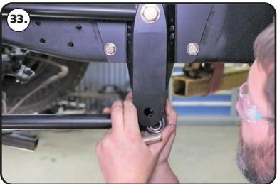
**33.** Insert (2) .625" ID x .740" long R-Joint spacers into the front R-Joint of each lower bar. The small diameter of the spacer goes into the R-joint. Insert the front lower bar R-Joint into the lower position of the frame mount.
