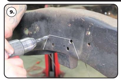
**9.** Drill the holes using a 1/2" drill bit. This will give the corner a round edge and eliminate the possibility for stress fractures
