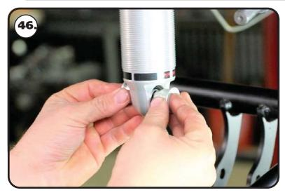
**46.** Insert the shock bearing t-bushings into the bearing of the shock body. The small outside diameter of the t-bushing will insert into the shock bearing.
