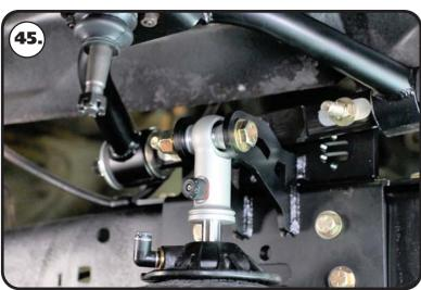
**45.** Install a 1/2" flat washer on a 1/2"-13 x 3" hex bolt. Insert the bolt/washer into the mount/shock. Install a 1/2" flat washer & 1/2"-13 nylok nut. Torque the hardware to 75 ft-lbs.
