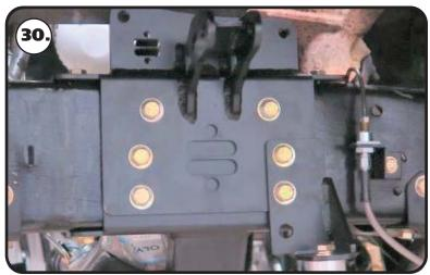
**30.** Install a 7/16" flat washer on each of (2) 7/16"-14 x 1 /4" hex bolts. Insert the bolt/ washers in the remaining bottom (2) bolts holes of the front (3) bolt holes. Install a 7/16" flat washer and 7/16"-14 nylok nut on the threads of the bolts. Do this for both sides. Snug the hardware, but do not torque the hardware at this time.
