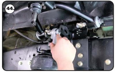
**44.** Insert the eyelet of the shock into the frame mount with the adjuster know toward the outside of the truck. Align the mounting holes with the through hole of the shock eyelet.
