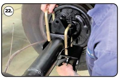
**22.** Install a supplied 5/8" u-bolt in each side of the upper bar mount. The u-bolts will nest in the slots of the upper mount. The U-bolts will run parallel to the axle tube.
