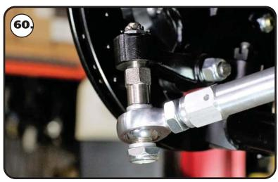
**60.** Install a 1/8" thick aluminum on the bottom side of the heim end followed by a 5/8"-18 thin nylok nut on the stud. Torque the nut to 45 ft-lbs.
