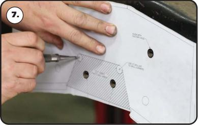
**6.** Use the template to center punch the corner holes of the area that needs to be cut out.
