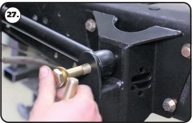
**27.** Line the through hole of the R-Joint with the of holes of the frame mount. Install a 5/8" flat washer on to a 5/8"-18 x 3 1/2" hex bolt, insert into the lined up holes. Install a 5/8" flat washer followed by a 5/8"-18 nylok nut. Repeat on both sides and tighten the bolts/nuts enough to eliminate any gaps.
