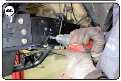
**33.** Drill the (4) holes for the front & rear side frame mounts using a 7/16" drill bit.
