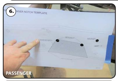
**5.** Cut the indexing holes out of the template and align them with the holes in the frame. We recommend taping the c-notch to the frame to hold it in position.
