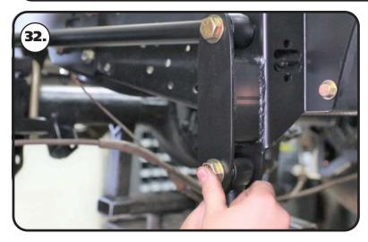
**32.** Line the through hole of the R-Joint with the of holes of the front frame mount. Install a 5/8" flat washer on to a 5/8"-18 x 3 1/2" hex bolt, insert into the lined up holes. Install a 5/8" flat washer followed by a 5/8"-18 nylok nut. Repeat on both sides and tighten the bolts/nuts enough to eliminate any gaps.
