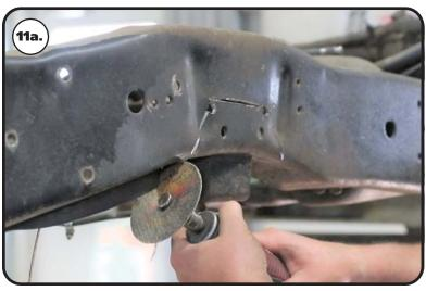
**11a & 11b.** Cut the notch with a saw-z-all, cutoff wheel, or plasma cutter. Grind all edges smooth. Cut the sides of the frame and across the bottom of the rail. The cuts on the bottom of the frame rail will be parallel with each other. The side frame cuts will blend into the drilled holes. The section of frame will fall out when cutting is complete.
