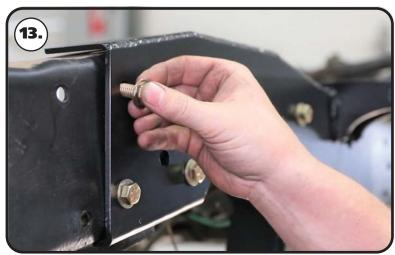
**13.** Install a 7/16" flat washer on each of (8) 7/16" x 1 1/4" bolts. This hardware gets installed in the sides of the c-notch. Install a 7/16" flat washer and 7/16" nylok nut on each bolt sticking through the frame. Tighten all of the c-notch side bolts. Tighten the hardware snuggly for the time being.
