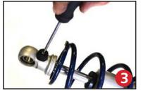
Before the upper spring mount can be installed screw the adjuster knob on the upper eye mount to the firmest setting (clockwise) as seen in figure 3. Then remove the Knob by holding it while removing the center screw.
