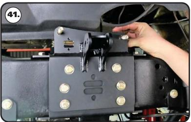
**41.** Install a 7/16" flat washer on each of (2) 7/16"-14 x 3" hex bolts. Insert a bolt/washer in each bottom (2) upper control arm mounting holes.
