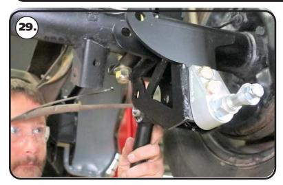
**29.** Insert (2) .625" ID x .740" long R-Joint spacers into the R-Joint of one end of each lower bar (23 5/8"). The small diameter of the spacer goes into the R-joint. Insert the rear lower bar R-Joint into the lower bar mount built into the axle mount.
