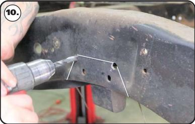
**10.** Drill the holes using a 1/2" drill bit. This will give the corner a round edge and eliminate the possibility for stress fractures
