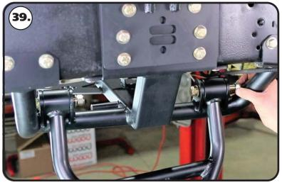
**39.** Install a 1/2" flat washer on each of (2) 1/2"-13 x 3 1/2" hex bolts. Insert the bolt/washer in the aligned holes with the threads to the rear of the truck. Install a 1/2" flat washer & 1/2"-13 nylok nut on the threads of the bolts. Re peat on the passenger side control arm. Torque the mounting bolts to 75 ft-lbs.
