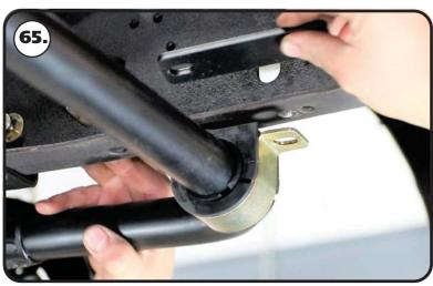
**65.** The sway bar includes a backer plate that needs to be installed on the top side of the frame flange. Align the backer plate holes with the holes drilled in the frame.
