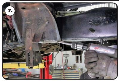
**7.** Remove the side and bottom rivets from the frame mounts.
