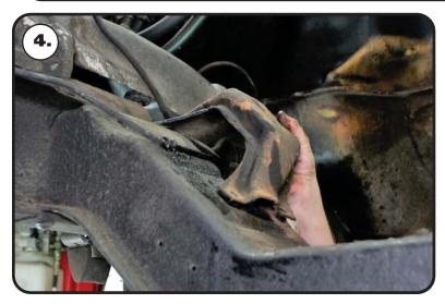
**4.** Remove the OEM engine mount stands.
