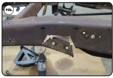
**11b.** The section of frame will fall out when cutting is complete.
