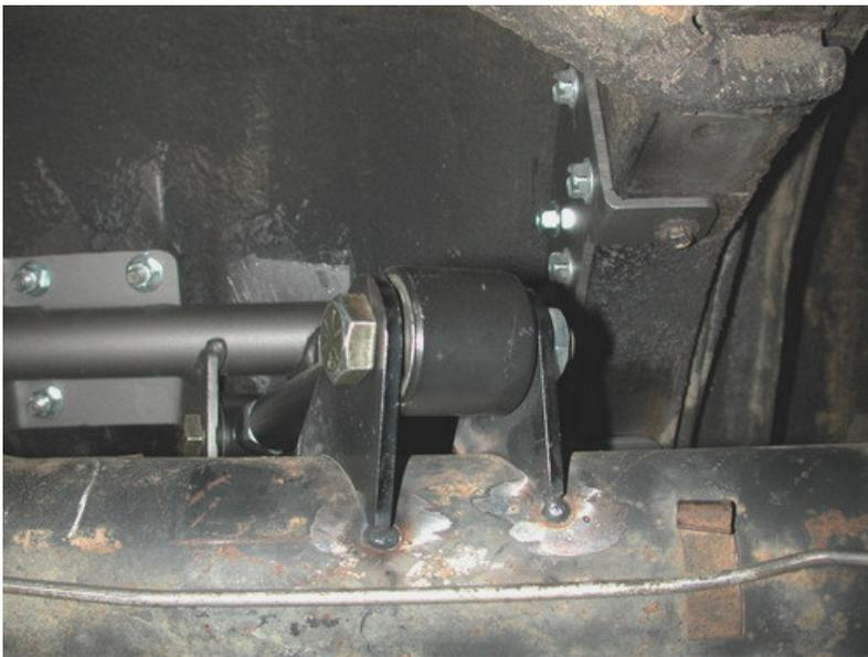
14. Once pinion angle, axle center and ride height are double-checked the tabs can be tack-welded to the axle. Then remove the bar (to avoid frying the bushings) and weld the tabs solid. Weld 1" at a time and skip around to avoid warping the axle. Reattach the bar to the axle.
