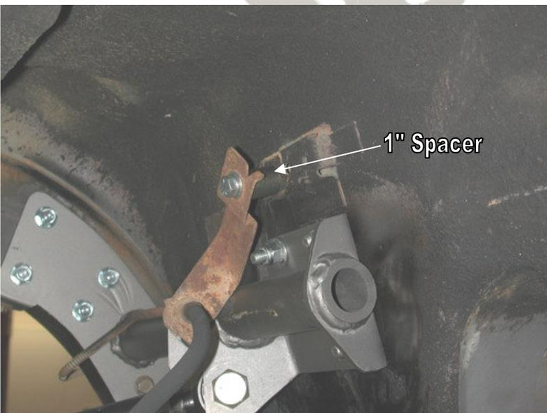
18. Insert a 5/8" x 4" bolt through the upper mount and Shockwave eye. There should be a 5/8" flat washer on each side of the poly bushing and one next to the head of the bolt. Fasten the assembly with a 5/8" Nyloc nut.
