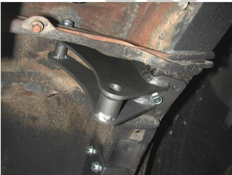
15. Attach the upper Shockwave mount to the factory upper shock mount using a  $\frac{1}{2}$ " x  $2\frac{3}{4}$ " bolt, Nyloc nut, and flat washers. Swing the bracket out to the frame rail to mark and drill 5 holes in the frame with a  $\frac{5}{16}$ " bit. Fasten with  $\frac{3}{8}$ " x 1" thread forming bolts and flat washers.
