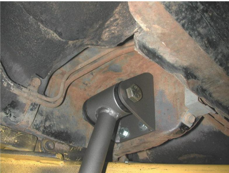
9. Bolt the new front lower bar mount to the body using 4  $\frac{3}{8}$ " x  $1\frac{1}{4}$ " bolts, 8 flat washers and 4 Nyloc nuts.
