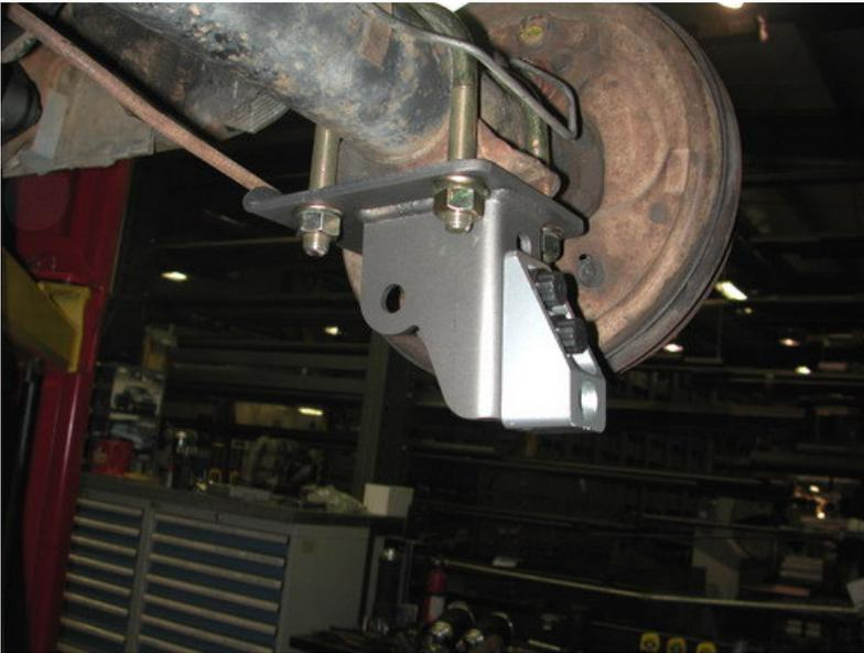
7. Using the supplied U-bolts, fasten the lower axle bracket to the factory leaf spring pad.
