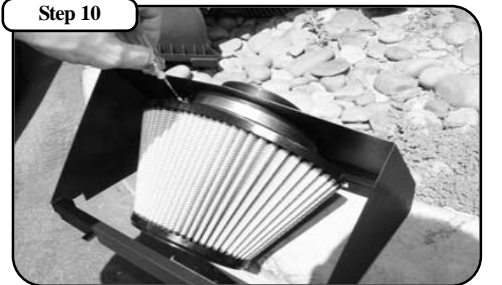
Place aFe air filter onto the air filter adapter. Tighten the clamp loosely for now just to hold the filter on. You will still need to rotate the filter.
