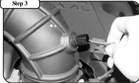
Disconnect the tempature sensor by sliding back the red clip, then pushing the black release tab and pulling off.
