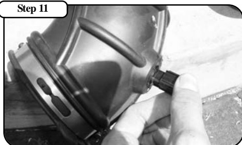
Remove the tempature sensor from the stock intake tube.
