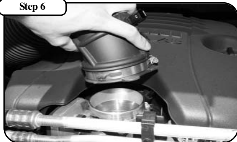
Pull up on the stock intake tube to remove it from the throttle body.
