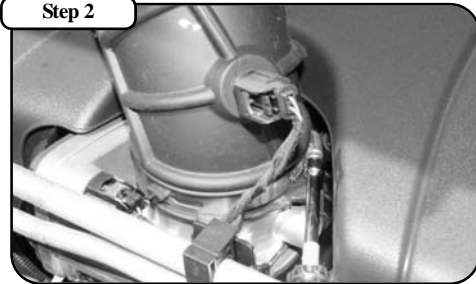
Loosen the clamp at the throttle body.
