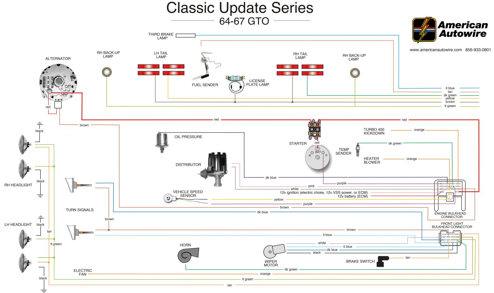
NOTICE: This schematic drawing is for <u>reference only</u>. Do not use the schematic to install this wiring kit! Use the instruction sheets included in each bag, which includes directions for proper terminations, and specific applications.
