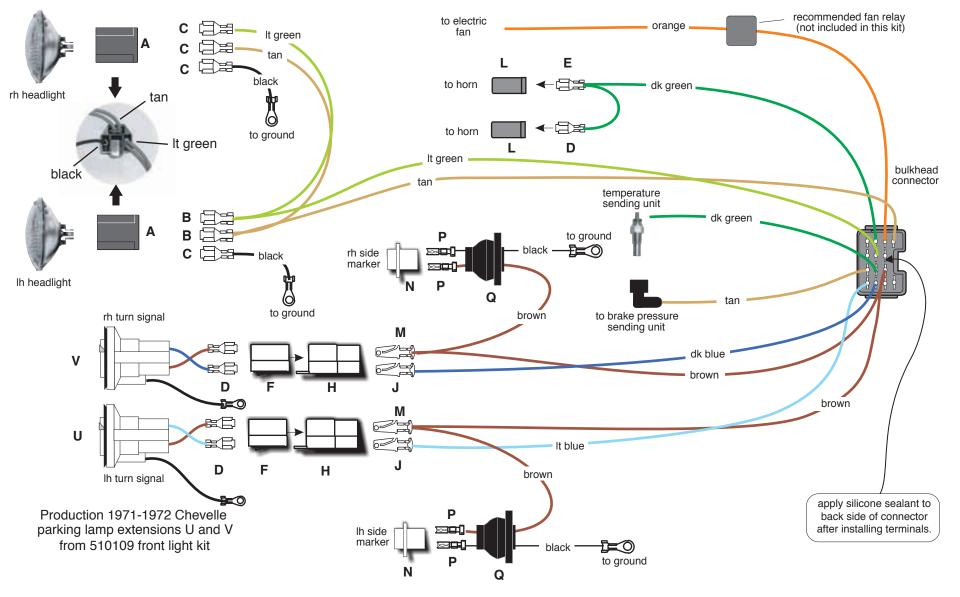
1. The 1972 Monte Carlo Front Lamp harness assembles basically like a combination of the 70 and 71-72 Chevelle assemblies found on sheets 2 and 4 of the production 510109 Chevelle instructions. No extra parts are needed. Only items from the production 510109 kit will be used in this assembly.
