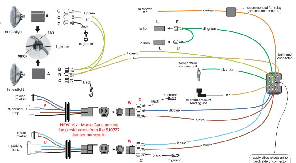
1. The 1971 Monte Carlo Front Lamp harness was very unique in that it utilized a parking and side marker lamp extension harness to complete the circuitry. If your car is a 1971 model, we have provided parking and side marker lamp extension harnesses U and V along with terminals and connectors C and W found in the 510337 Jumper harness kit to aid you in the completion of your front lamp connections. The balance of the 510109 front lamp kit installs the same as a 1971 Chevelle.
