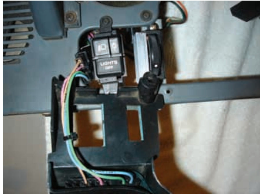
LH indicator lamp extension, Item A, is shown above with the dash insert flipped down and the extension plugged onto the circuit board pins along with the mating end of the extension plugged into the dash connection.
