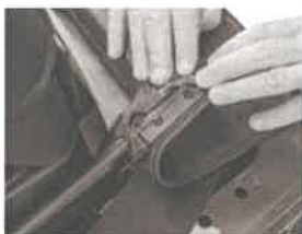
Peel back foam to expose two screws which need to be removed. Save the screws
