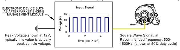
Refer to above Example 5, for use with the Fuelab Electronic Fuel Pressure Regulator, Models 52901 and 52902, that creates its own pulsed signal. These regulators automatically control the fuel pump, without the use of switching means or other components such as described in examples 2 and 3. Refer to instructions for the Electronic Regulator, for proper wiring and installation.
