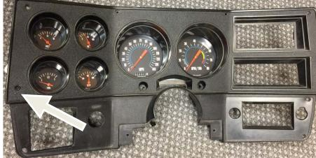
b. Due to differences in dash bezels from year to year, the upper aluminum standoffs are adjustable. Loosen these from the cluster and adjust them to fit the bezel. Use the black screws provided to secure the bezel to the aluminum standoffs.
