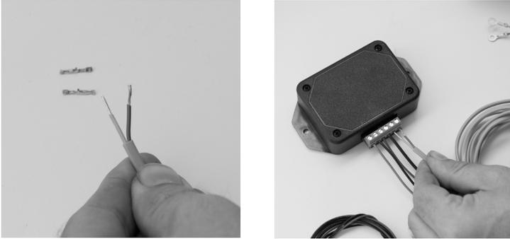
1. The thermocouple wires from the pyrometer probe are to be connected to terminals #5 and #6. Strip 1/8" to 3/16" insulation from each wire of the probe harness. Connect the Yellow wire to #5, and the Red wire to #6.
