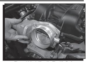
Figure 12 Installing the Throttle Body.
