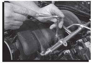
**Figure 5 Removing the Intake Retainers.**
