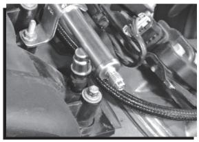
**Figure 2 Schrader Valve Location.**
