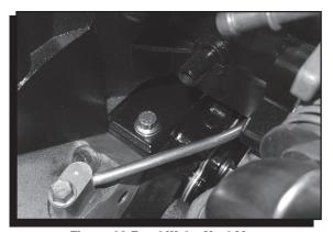
**Figure 13 Front Water Vent Line.**
