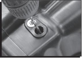
Figure 6 Drilling the MAP Sensor Hole.
