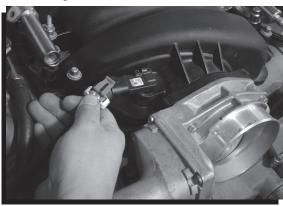
Figure 3 Disconnect Sensors and Remove the Throttle Body
