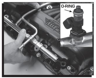
Figure 9 Fuel Injector and Rail Installation.
