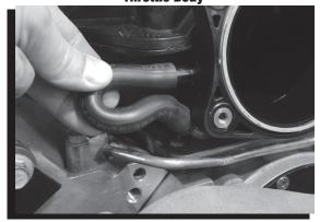
**Figure 4 Mark and Remove Vacuum Lines.**
