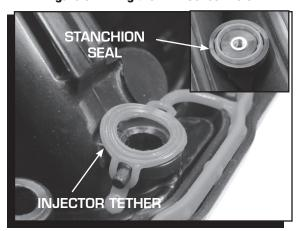
**Figure 7 Intake Seals and Injector Tether.**
