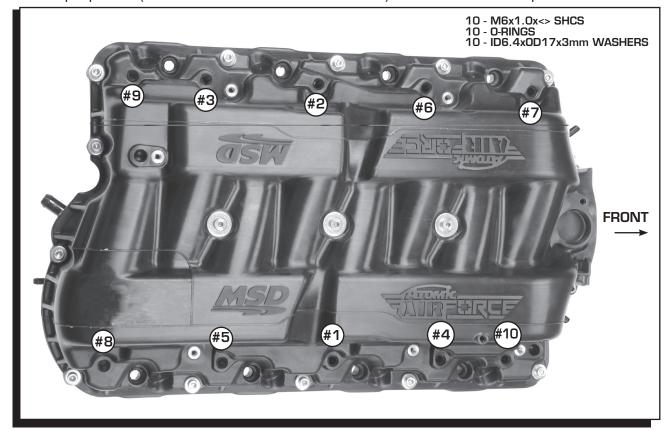
Figure 11 Intake-to-Cylinder Head Torque Sequence.
