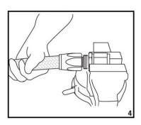
5. To complete the assembly it doesn't matter whether the nipple or the socket is held in the vise. Holding one or the other in the vise and using a suitable wrench on the other, tighten the socket onto the cutter threads until the socket is within .060" of bottoming on the nipple. Do not use an adjustable or over-size wrench or you will damage either the nipple or the socket.
