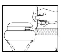
2. Place the socket in a vise and insert the end of the hose into the socket until the hose butts against the bottom of the threads. Gently pull the hose back until there is a 1/16" to 1/8" gap between the end of the hose and the bottom of the socket -mark hose at bottom of socket with a felt pen so that you can detect any tendency of the hose to be pushed out as you complete the assembly.
