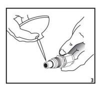
3. Lubricate the inside of the hose, the nipple threads and the socket threads with Earl's Assembly Lube or Engine OII. Place the nipple in a vise.
