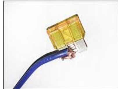
Wire Jammed Into a Fuse
