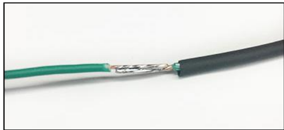
Soldered Connection w/ adhesive heat shrink
