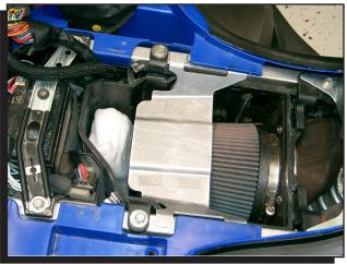
Figure 2 Hook Bracket and Velcro Install.
