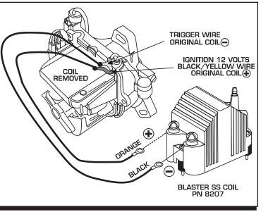
Figure 2 Wiring with a Blaster SS Coil.
