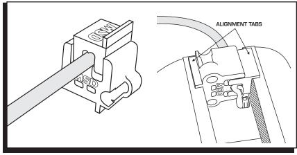
Figure 9 Crimping the Terminal.
