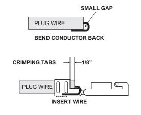
Figure 7 Positioning the Wire in the Terminal.
