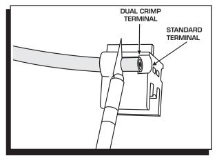
Figure 5 Stripping the Sleeve.
