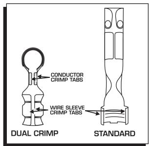
Figure 4 Identifying the Different Style Terminals.
