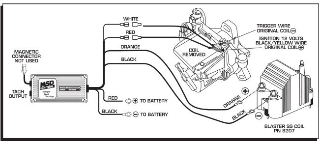
Figure 3 Wiring an MSD SCI Ignition with a Blaster SS Coil.
