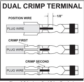
Figure 8 Crimping a Dual Crimp Terminal
