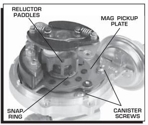
Figure 11 Removing the Vacuum Canister.
