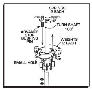
Figure 7 Locking Out the Advance.
