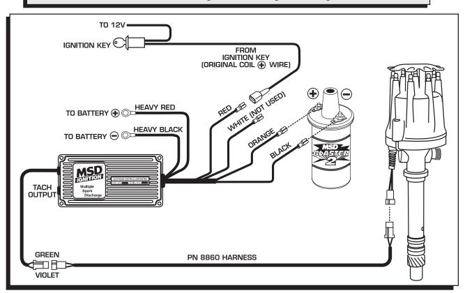
Figure 13 Wiring to an MSD 6-Series Ignition Control.
