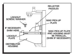
Figure 12 Checking Installation of the Lockout Plate.
