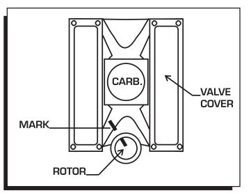
Figure 8 Marking the Rotor Location.
