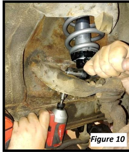
10. Using a spanner wrench (Part number T114W or T115W), adjust the spring seat adjuster to set the ride height of the car. Raising the spring seat will raise the ride height. Lowering the spring seat will lower the car. If you have not done so, lubricate the threads on the shock with anti-seize prior to making any ride height adjustments.
