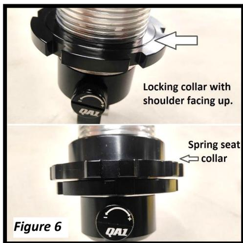
1. Screw the aluminum lock nut (shoulder up) and the spring seat adjuster nut (shoulder up) down to the last thread - NO FURTHER. **(Figure 6)** Now is a good time to lubricate the threads of the shock with **Permatex® Anti-Seize lubricant**.
