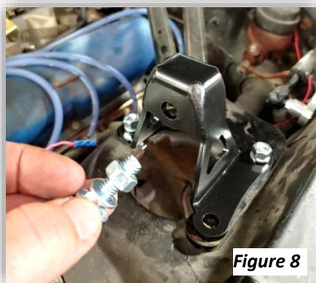
5. Install the new shock tower cap included in the kit using the factory hardware. **(Figure 8)** Torque to 26 lb.-ft.
