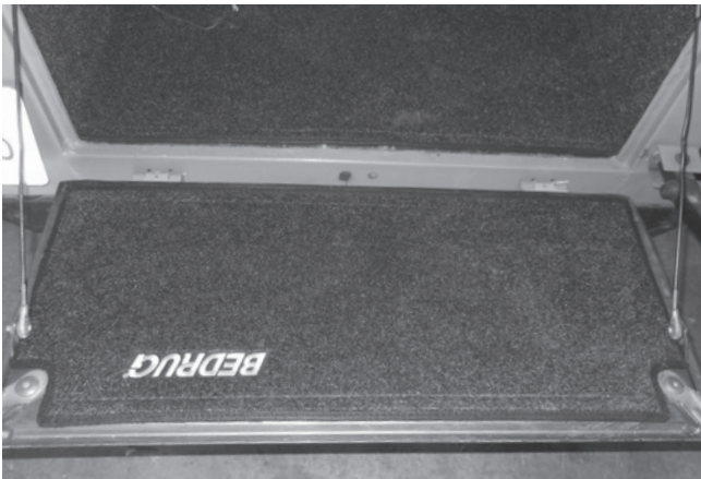
COMPLETED TAILGATE INSTALLATION
