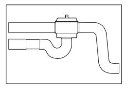
Before re-installation, the air injection tubes must be modified as shown above using the hose and clamps provided in the kit.
