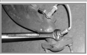
Remove the front driver side oxygen sensor from the manifold.
