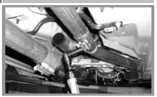
Separate the cat-back system by loosening the 2 nuts on each band clamp and prying the locking tabs up with a small screwdriver while sliding the clamp towards the rear of the car.
