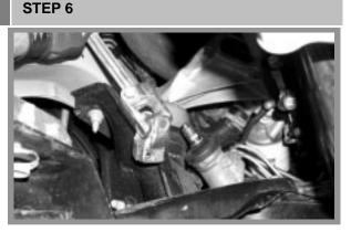
• Remove the bolts from the top and bottom of the steering shaft and remove the shaft. You may find more working space by removing the motor mounts from the engine by removing the nuts that secure the mounts to the K-Member and carefully jacking the motor up and supporting it with a block of wood, then removing the fasteners that attach the mounts to the engine block. DO NOT ATTEMPT TO LIFT THE ENGINE BY JACKING UNDER THE OIL PAN.
