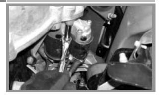
Unbolt and remove the starter from the bell housing.
