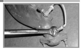
Remove the front driver side oxygen sensor from the manifold.
