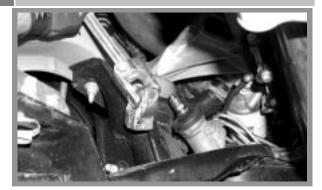
Remove the bolts from the top and bottom of the steering shaft and remove the shaft. You may find more working space by removing the motor mounts from the engine by removing the nuts that secure the mounts to the K-Member and carefully jacking the motor up and supporting it with a block of wood, then removing the fasteners that attach the mounts to the engine block. DO NOT ATTEMPT TO LIFT THE ENGINE BY JACKING UNDER THE OIL PAN.
