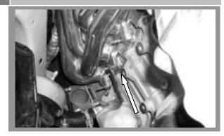
Remove the bolt that secures the dipstick tube to the driver side cylinder head and pull the dipstick tube straight up to remove it from the engine.
