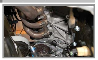
Place a jacking device under the bell housing and remove the driver side motor mount from the engine. This will give you access to the bottom row of header nuts.
