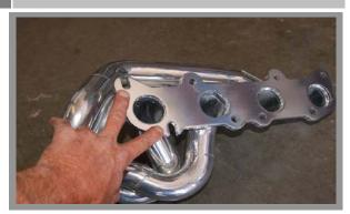
• Looking at the BBK Header Flange, remove the studs that correspond with the notches in the flange. On the driver side it's the two most rear studs. Those will be replaced with supplied bolts. <u>NOTE!!!</u> There are 2 thread pitches supplied because the manufacturer changed the thread pitch used after 2011. You will have to compare the supplied bolt to the factory stud to confirm which thread pitch to use.
