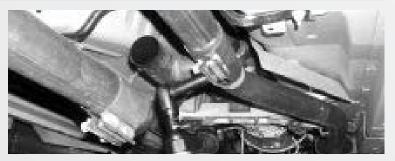
Separate the cat-back system by loosening the 2 nuts on each band clamp and prying the locking tabs up with a small screwdriver while sliding the clamp towards the rear of the car.
