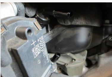
Remove factory PCV hose behind throttle body, now assemble oil separator kit as shown on front page. Make sure to hook up hose from the draw side of the oil separator to the intake manifold.
