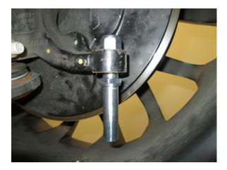
**Step 6** If the vehicle is at stock ride height then slide the tie rod end over the straight shank of the bottom of the tie rod stud then install the appropriate amount of spacers for tightening. If the vehicle is lowered you are going to want to install the appropriate amount of spacers between the spindle and rod end to achieve the measured angle from step 1, and then install the appropriate amount of spacers for tightening.
